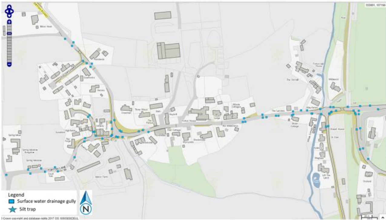
Figure 44: Highways Surface water drainage in Forton.
